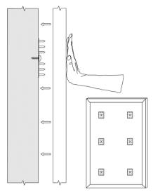
The use of construction adhesive to secure the panels is recommended
